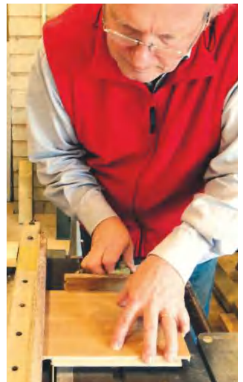
▲ Pic.4 Creating the lap joint using the table saw
